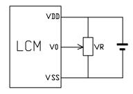
$V_{\text{DD-}}V_0\text{: LCD Driving voltage}$
